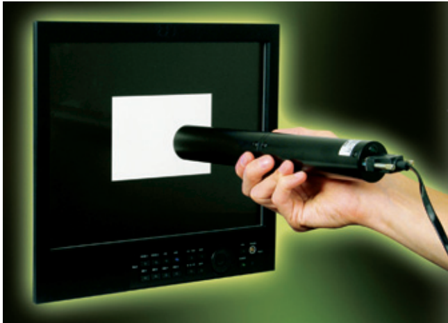
Measuring of white balance on an LCD monitor by use of DK-Technologies LCD colour sensor.
