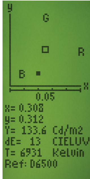
The CIE display showing the measurement as x,y coordinates. The solid ball is the actual measurement, while the square is the target.
